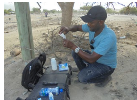
Testing the well water for pH, TDS and EC to check on level of service improvements
