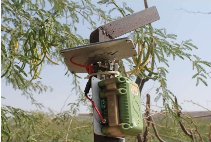
Left: SweetSense sensors placed near a rehabilitated borehole to detect functionality and water flow. Right: The Afar region customized web-based platform that provides real time functionality monitoring for the RWB and WWOs, allowing for better decision-making at the regional level
